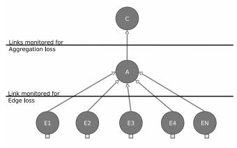
N Edge Nodes with traffic generators attached
