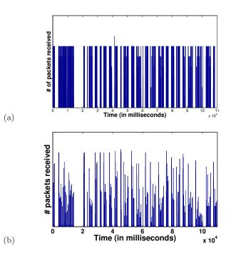
Figure 5: Pictorial proof of ON/OFF characteristics: Time series of data center traffic (number of packets per time) binned by two different time scales. Traffic in figure (a) is binned by 15ms and by 100ms in (b).
