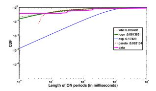
Figure 8: CDF of the distribution of the ON period lengths at one of the switches in DC10. The figure contains best fit curve for lognormal,weibul, pareto, and exponential as well as the least mean errors for each curve. We notice that the lognormal fit produces the least error
