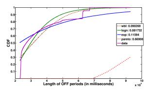
Figure 7: CDF of the distribution of OFF period lengths at one of the switches in DC10. The figure contains best fit curve for lognormal,weibul, pareto, and exponential as well as the least mean errors for each curve. We notice that the lognormal fit produces the least error
